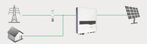
In this system, the inverter output will adjust to match the load consumption power continuously to restrict the export power.
